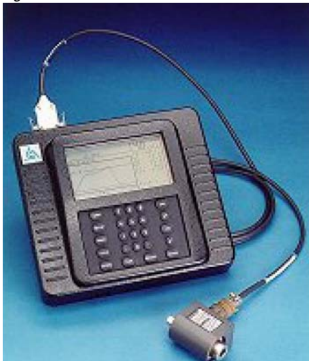
Figure 27. Two-Channel Transient Recorder
